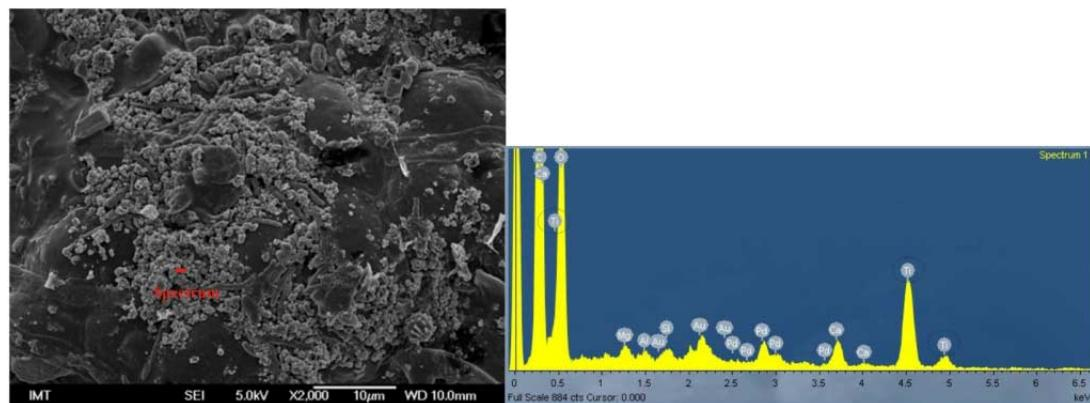
Fig. 2. (a) Nano-TiO<sub>2</sub> dispersed over the lower leaf surface to give a final concentration of 5,000 µg/g dry weight leaf. The red spot indicates where the spectrum for energy-dispersive X-ray spectroscopy analysis was performed (EDS) (b), to confirm the presence of Ti.
