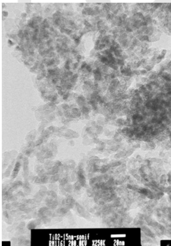
Fig. 4. Transmission electron microscopy of tested nanosized TiO<sub>2</sub> particles, showing their shape and size.
